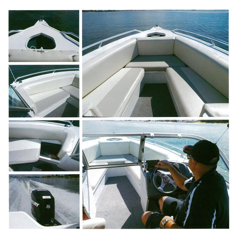
upholstered with a deep backrest. There's plenty of stowage underneath the seat cushions and there is an option of a table, with sockets to situate it in either the bow lounge or aft in the cockpit. A tonneau cover for the bow lounge is also on the options list.
